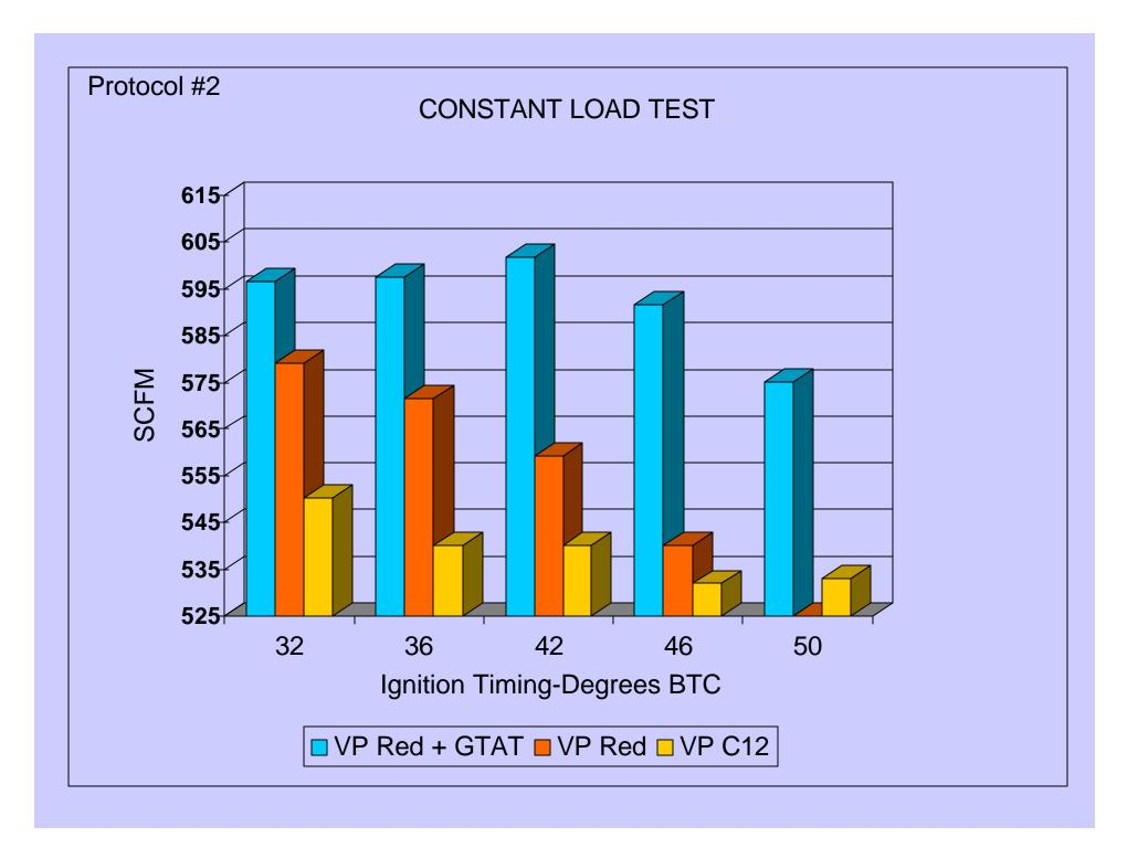
8. VP Red+GTAT had superior performance to the higher octane VP C-12 under all test conditions in the constant load test.
