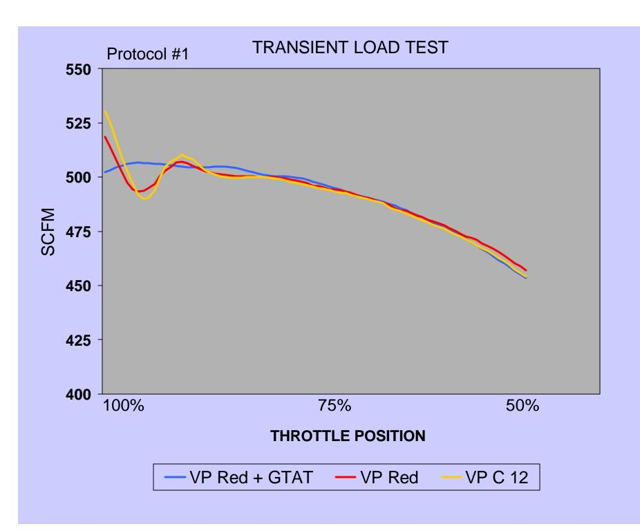
7. VP Red+GTAT had greater stability than untreated VP Red under increasing thermal and pressure stresses as ignition timing was advanced.
