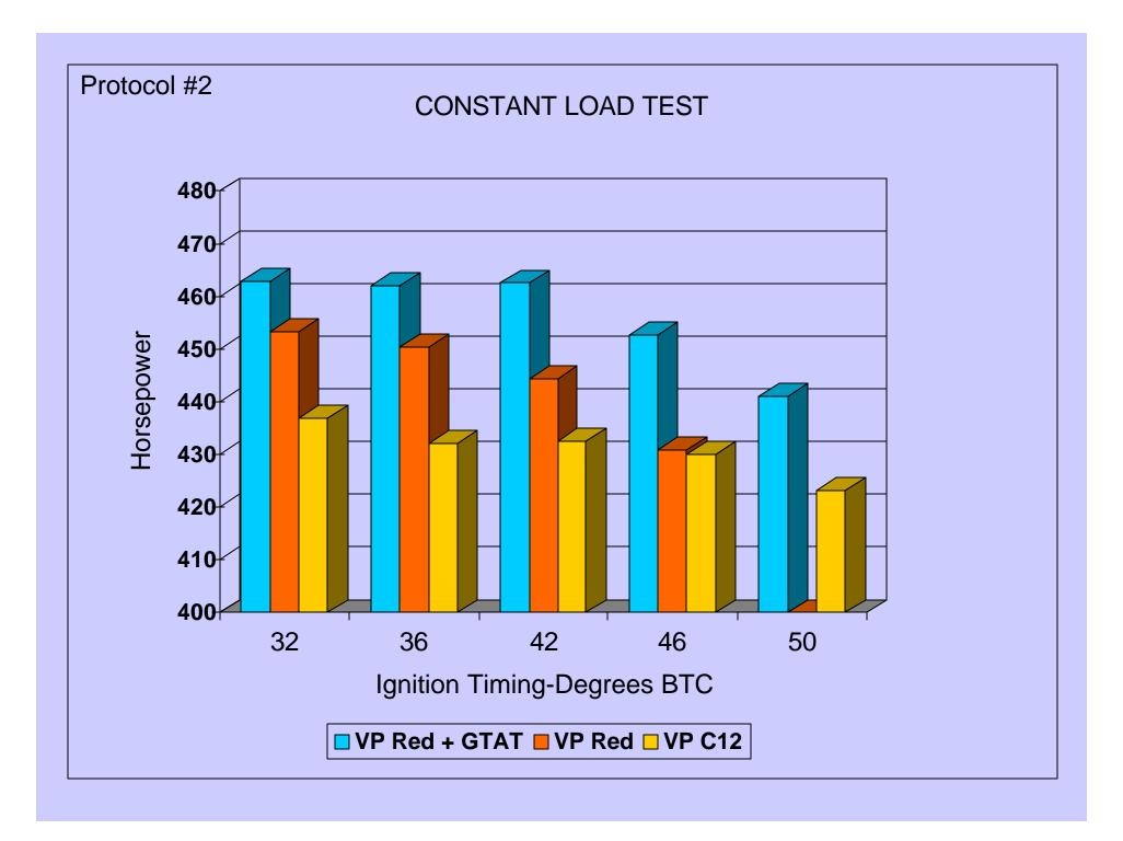
2. In the constant load test Red+GTAT had greater volumetric efficiency than the untreated fuels and the difference increased with spark advance.
